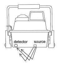
The Geiger Mueller detector inside the meter measures the amount of gamma radiation reflected, or "scattered back", from the material in terms of counts per minute (CPM).
